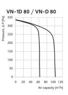
The abrupt curves show high pressure performance of VNV fans and constant air flow while operation of many fans integrated into single ventilation shaft:
