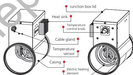
The temperature control knob with temperature range from -10 °C up to +40 °C is placed on the junction box front panel. The NK...U heater is equipped with a built-in temperature sensor located inside of the air duct.
