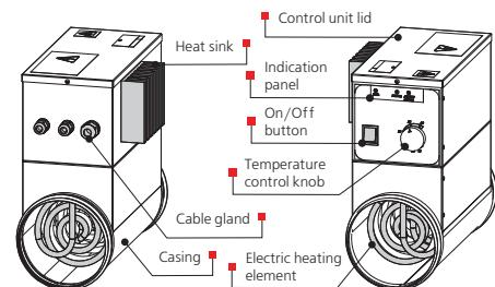
The NK...U model with a control unit is equipped with a triac power control unit. Power control is effected by means of switching on/off the maximum load commutated by the semiconductor device that is free of any mechanical wear parts. The load commutation starts at zero current and load to disable any magnetic field interferences.
